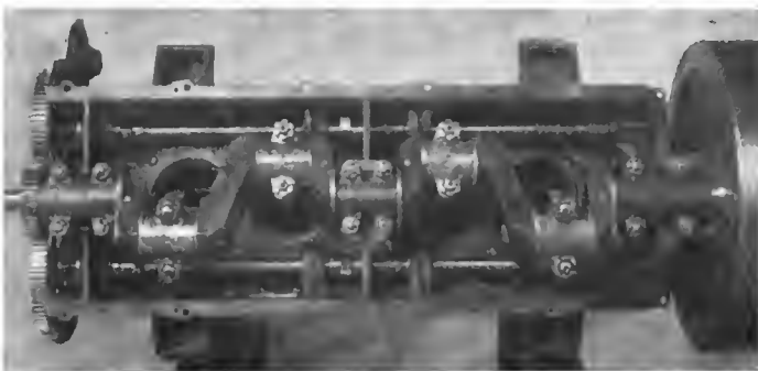
UNDER SIDE OF MOTOR SHOWING CRANKSHAFT DETAIL.
